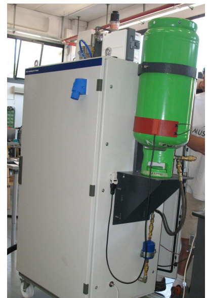
Heated Refrigerant Supply with Tank Support
